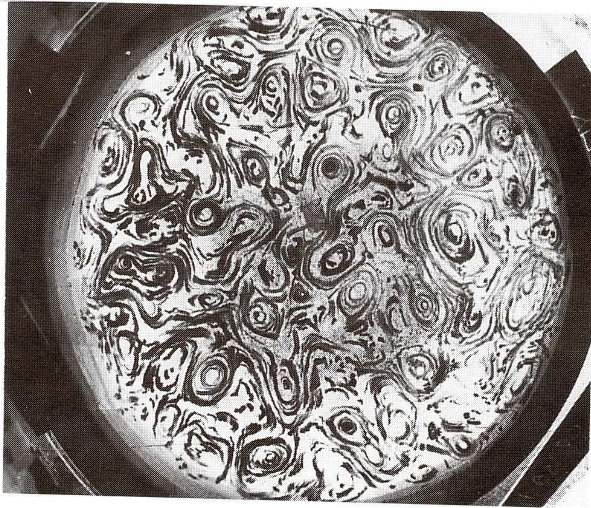
Figure 17: An example of irregular convective vortex pattern; Ra_f = 2.0 \cdot 10^8 , Ta = 7.1 \cdot 10^7 . (After Boubnov & Golitsyn, 1986, courtesy of Cambridge University Press).
