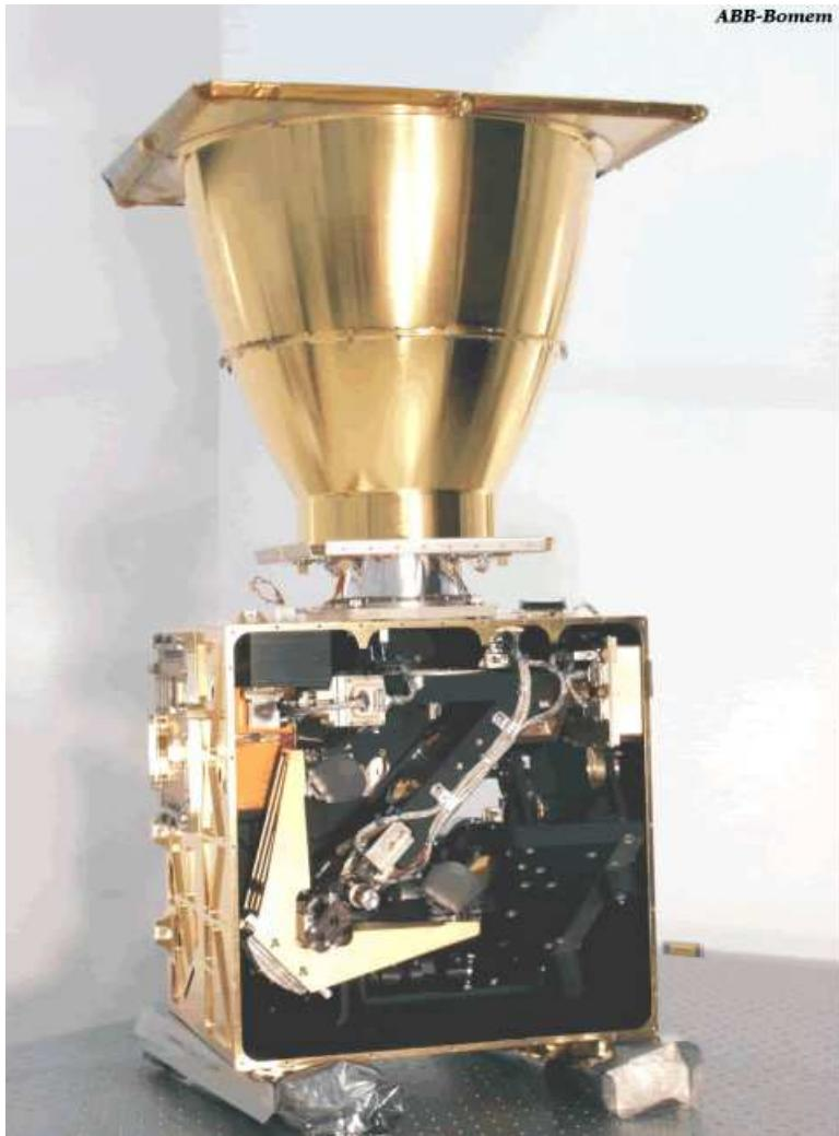
The ACE-FTS is the main instrument on SCISAT-1. It is a high spectral resolution ( $0.02\text{ cm}^{-1}$ ) Fourier Transform Spectrometer (FTS) operating from  $2.2$  to  $13.3\text{ }\mu\text{m}$  ( $750$ - $4400\text{ cm}^{-1}$ ) with a Michelson interferometer that was custom designed and built by ABB-Bomem in Quebec City.
