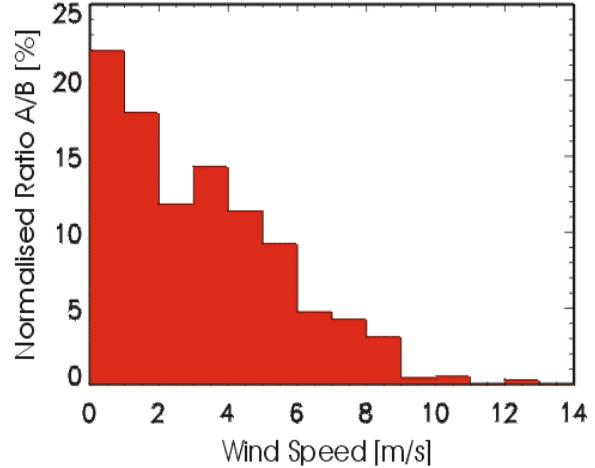
Any oil pollution in the three CS test sites is visible only at wind speeds up to 9-10 m/s !
