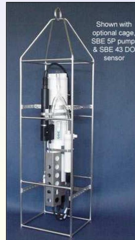
Shown with optional cage, SBE 5P pump, & SBE 43 DO sensor
